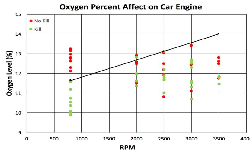
Figure 6. Successful engine stalls are indicated by green dots and unsuccessful stalls are represented by red. The black tend line indicates our projected stall rates from higher RPMs (from 3000-3500RPM). The line is extrapolated with the assumption that a larger bag would allow for successful engine stalling.
